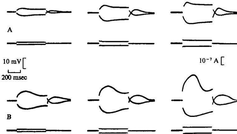
Fig. 5. Two examples of the effects of intracellular currents (lower traces) on the myocardial membrane potential at rest (upper traces). (A) the membrane displays a 'normal' rectification associated with a weak delayed rectification. (B) (other preparation): presence of a graded active response of the membrane during the application of depolarizing pulses. Distance between internal stimulating and recording electrodes, about 100 μm.
