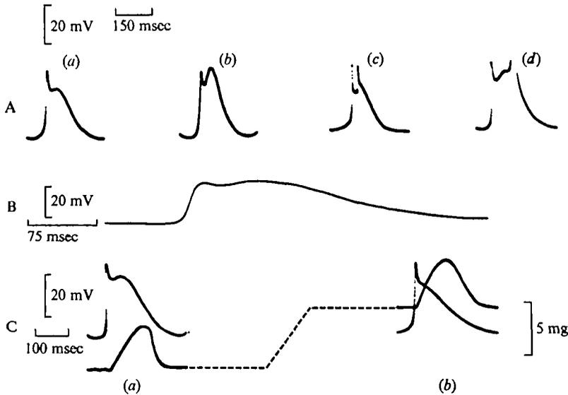
Fig. 2. (A) Various types of intracellular electrical responses recorded in the myocardium. (a, b) Most common responses. (c, d) Two modifications occurring during the repolarization phase. (B) Electrical response recorded at a rapid sweep speed. (C) Effect of stretching the heart on the contour of the responses (mechanogram tracings connected by dotted line). (a) Recordings under usual conditions. (b) Recording after stretching.
