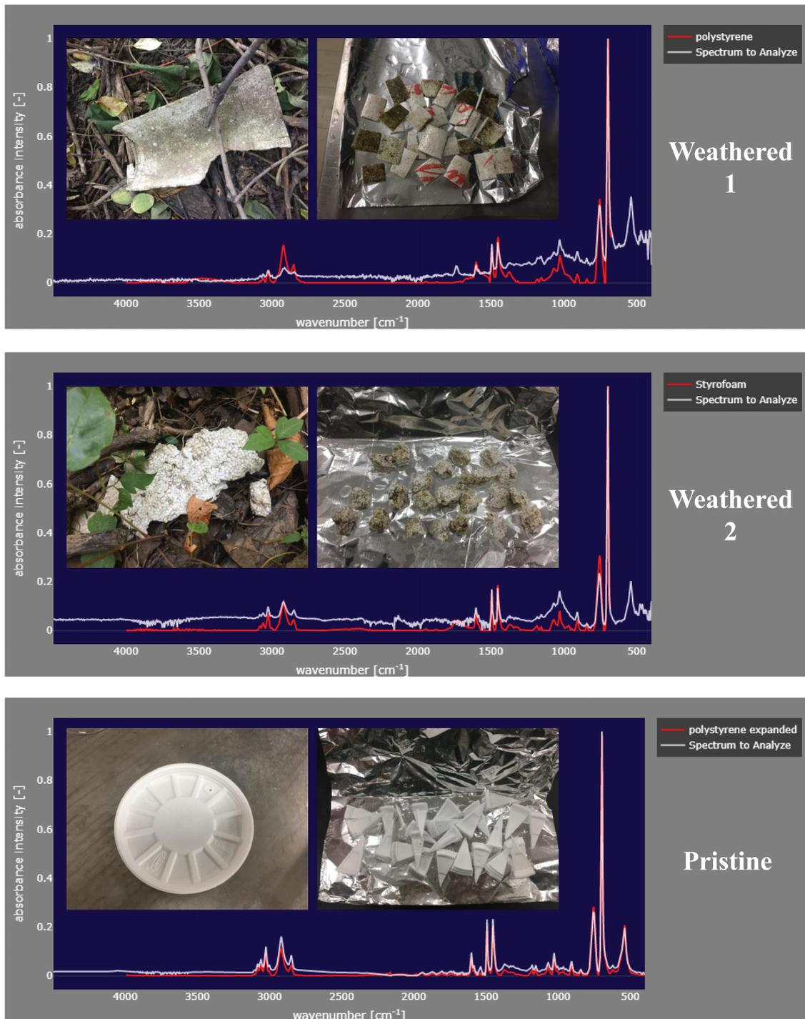
**Fig. 1.** Images of the original and cut pieces of the PS foam items comprising the three experimental treatments, with confirmatory ATR-FTIR spectra. Spectra in white represent our samples, spectra in red represent the closest spectral match obtained via OpenSpecy.
